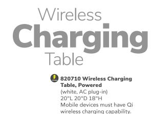
**Please Note:** Customer is responsible for providing labor and an electrical power source to the furniture. One 110V power source is required for each charging panel. Two charging units can be daisy chained together. 10A max per charging panel.
